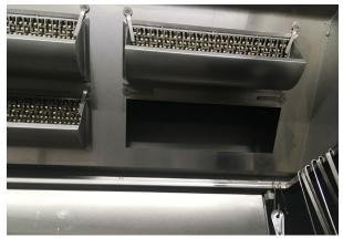
4) To clean place 2ea filters face down in the dishwasher and run the standard cycle
