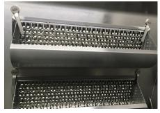
8) Remove any fat and grease from the rear wall sheet
